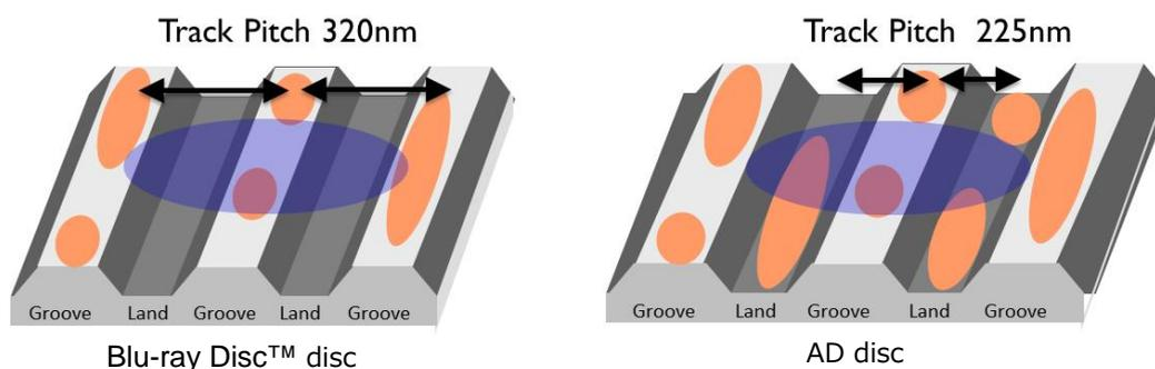
Figure 7. Land-and-groove recording
