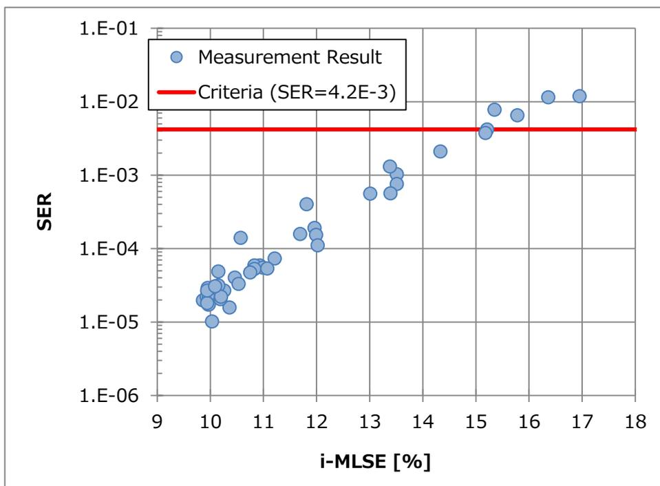
Figure 9. i-MLSE signal quality evaluation index and SER
