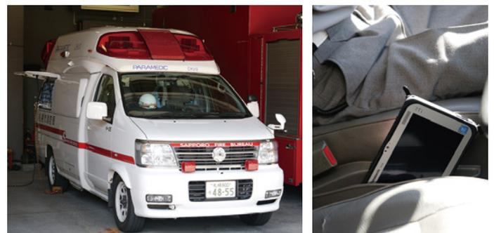
Toughpad FZ-B2, which is resistant to vibrations and both low and high temperatures, is always kept in the side of the passenger seat in the ambulance.
