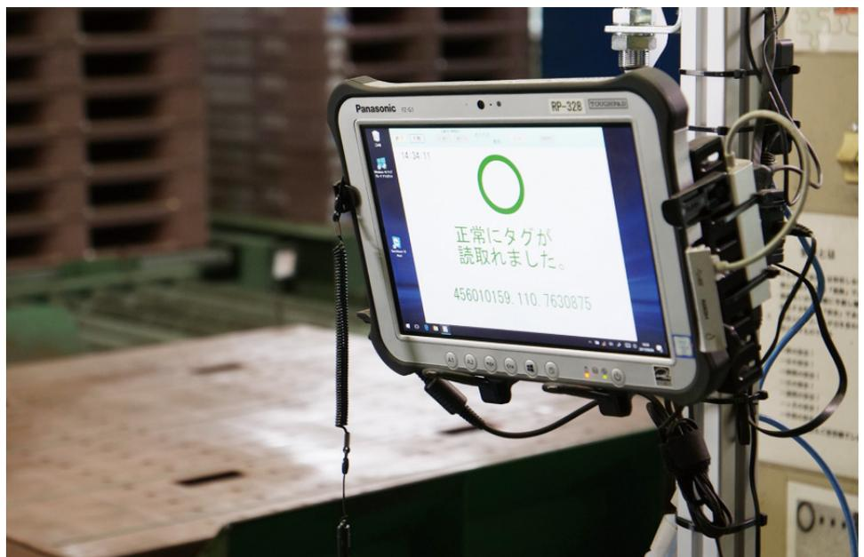
FZ-G1 is used to inspect the quality of RFID tags. Each RFID tag is read by sensors that are installed in the washing and cleaning line. The evaluation of whether or not radio frequencies are properly transmitted from the tags will be conducted on FZ-G1.
