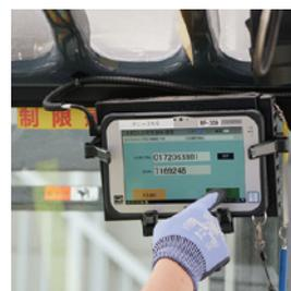
(Above image) The data of RFID tags attached to the pallets is read and uploaded via FZ-M1 to the data server while the pallets are placed on the forklift forks and are lifted and moved with the forklift.
