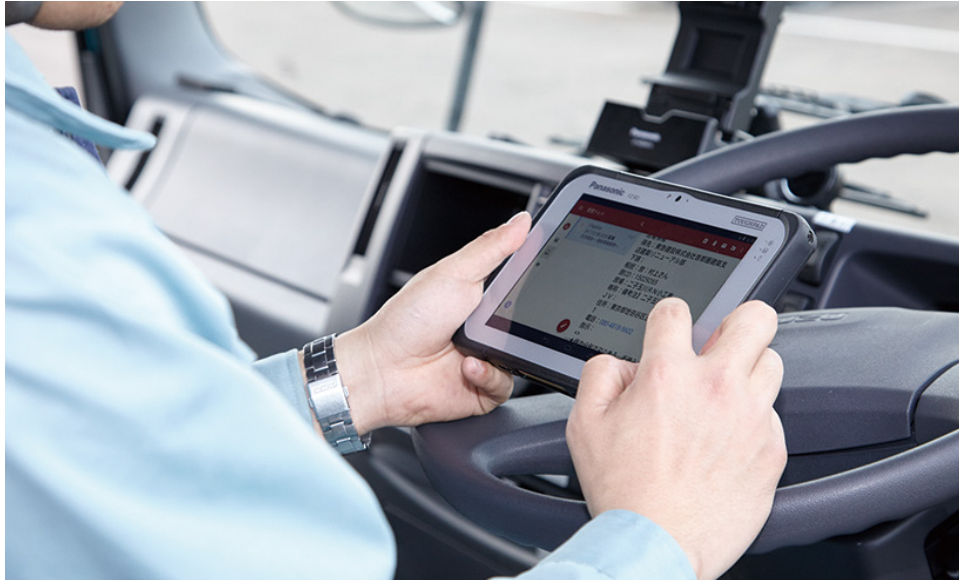
FZ-B2 enables users to easily check email messages and enter data into a daily report and into electronic manifest systems, while the user sits in the driver's seat in a parked truck. Some field workers operate the tablet with their gloves on.
