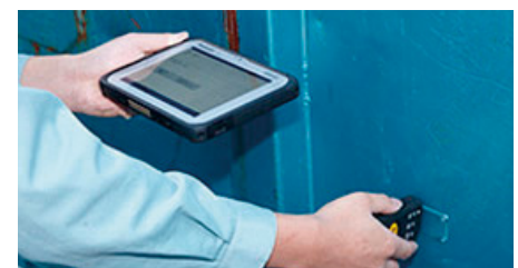
The In-metal Tags are attached to each one of the containers. Dedicated readers can be used to read the individual identification data of each container from the tags. The container data can be brought into sync with FZ-B2 through Bluetooth so as to easily reflect the data in the company's database.
