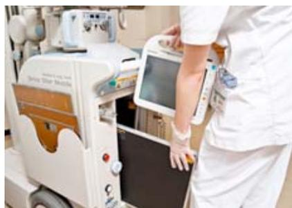
As the X-ray film cassette is extracted using the left hand, the barcode is read by the CF-H1 held in the right hand.
