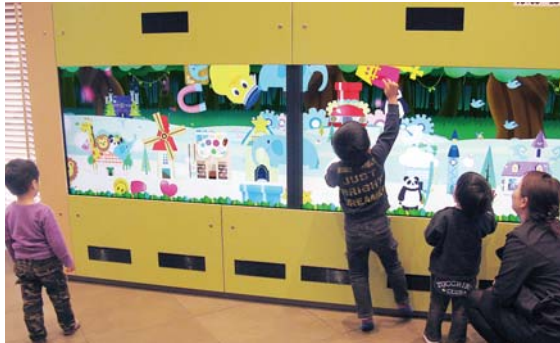
The display is installed at a height that enables children to touch the top of the screen.
