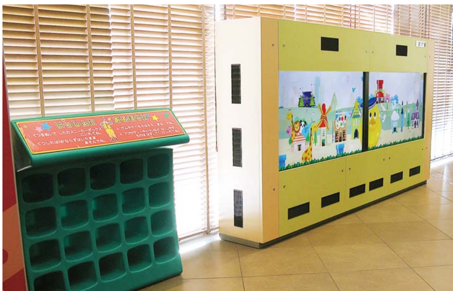
"Digital Playland" integrates two 65-inch displays, a PC for playing content, speakers, amplifier, etc. in a housing. It is also equipped with a cooling fan.
