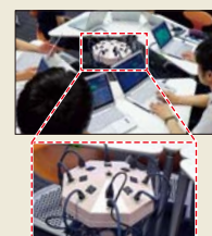
▲ A radial pole with 8 HDMI terminals. Gathers computer HDMI cables for easy movement.
