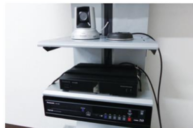
HDVC main unit installed in a mobile rack
