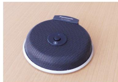
High sensitivity boundary microphone
