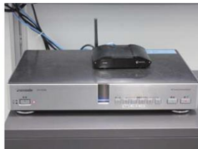
HDVC can connect to a PC wirelessly via WIVIA (distributed by Uchida Yoko).
