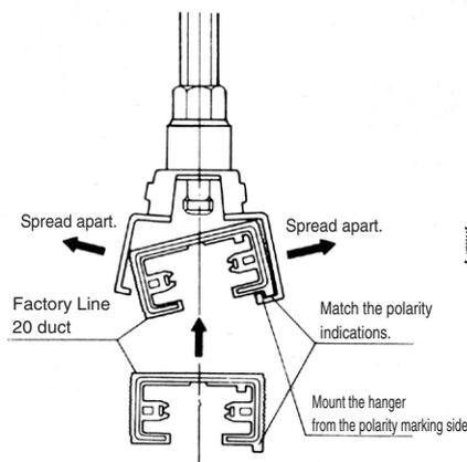
3. Fit the duct into the hanger, and then turn the cap to the right and tighten the securing screw in order to secure the duct.
