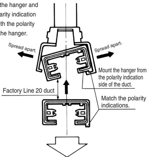
3. Fit the duct into the hanger, and then turn the cap to the right and tighten the securing screw in order to secure the duct.
