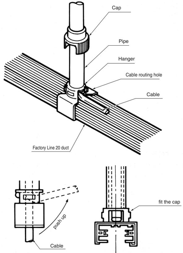
• Use single-conductor cables of 1.6 or 2.0 mm<sup>2</sup> in size.
