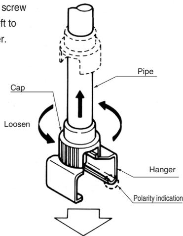
2. Spread apart the hanger and match the polarity indication on the duct with the polarity indication on the hanger.
