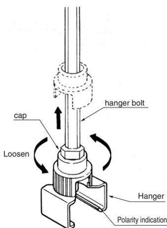
2. Spread apart the hanger and match the polarity indication on the duct with the polarity indication on the hanger.
