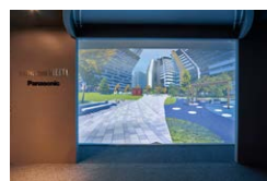
The image above is the "MIERVA Dome Type". An immersive experience can be obtained by calculating the viewer's point of view (standing position, height) and projecting images on a 1/1 scale. It is possible for multiple people to experience VR images at the same time, which could only be experienced by one person through conventional goggles.
