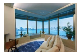
The image above is the "VIRTUAL STAGE MIERVA View Experience Type" that lets you experience the spectacular scenery from the windows with images. Images taken at a fixed point from the actual building are projected onto a screen outside the window using four high-brightness laser projectors and ultra short focus lenses.
